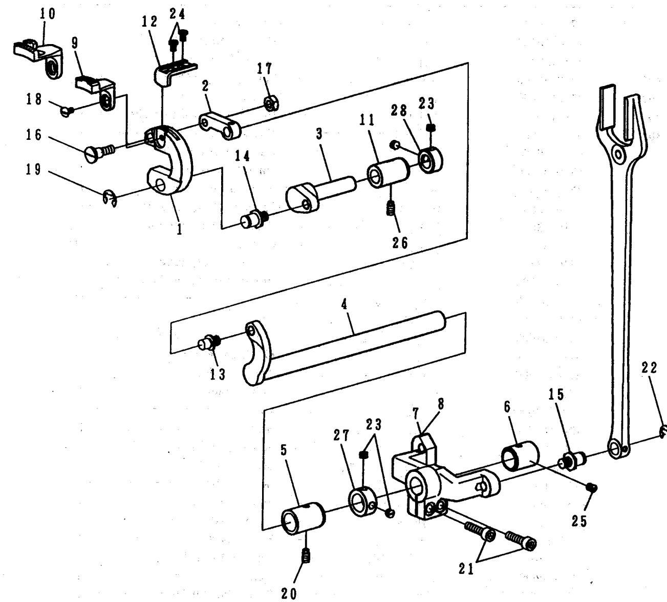
E. 送料机构 FEED MECHANISM COMPONENTS(1/2)
