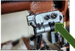
**STEP ONE:** Remove the two screws on the back of your machine, place the silver mounting bracket on the machine with the screw holes in line with the farleft side, then screw in the bracket firmly.
