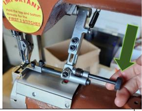
**STEP THREE:** To lower your guide to be in line with the needle, take your Allen keys provided to you, and turn these two screws COUNTER-CLOCKWISE to loosen, then pull down gently. To tighten screws, turn CLOCKWISE.
