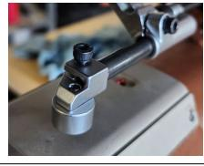
**STEP FIVE (Optional if you're sewing round edges):** To change from straight edge guide to round edge guide, remove the 2<sup>nd</sup> from edge screw, remove the flat edge, then put round edge guide onto the peg. and tighten the screw.
